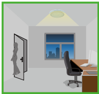
The light dims to stand-by period after hold-time and stays on selected minimum dimming level.
